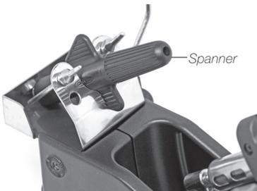
Use the spanner to remove and replace the tips.
