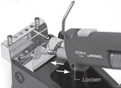
Place the Soldering Iron in the extractor and remove the tip.
